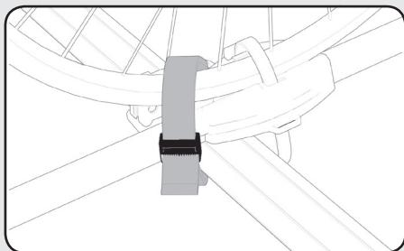
**For increased safety, fasten your bicycle to the carrier with the additional safety belt.**
